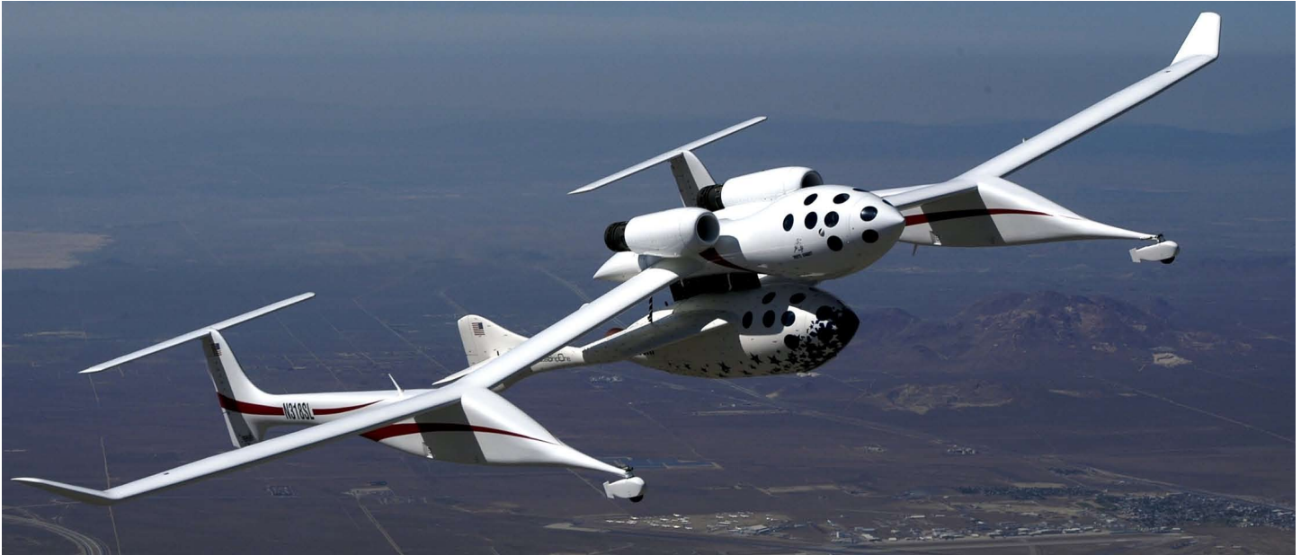
A specially-designed jet plane carried SpaceShipOne to 14 km before launching the 2004 X-Prize winner to its goal. Photo courtesy of Scaled Composites, LLC.
